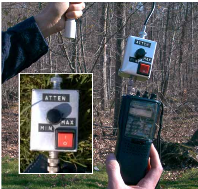
More Fox Hunt Equipment - NZ0I uses this clever "offset attenuator" to reduce the signal from the Fox when working in close. Details at www.qsl.net/nz0i
