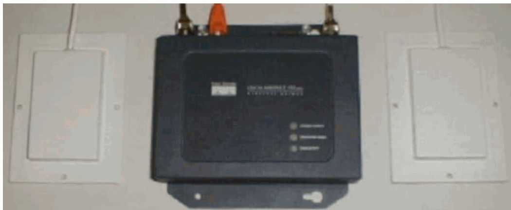
Figure 4 Cisco Aironet 350 Series Wireless Devices with Two 6.0 dBi Patch Antennas for Diversity
