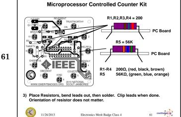
**Microprocessor Controlled Counter Kit**
