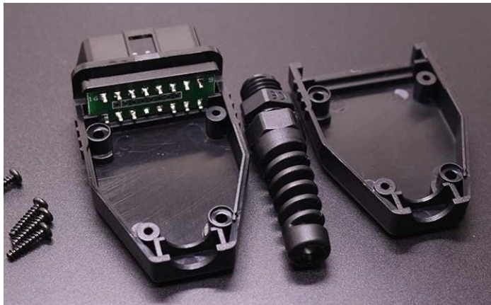
Figure 3. Open the connector and find pins 4 and 16
