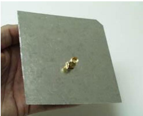
Solder the four ground legs on the front side. I found that clean galvanized steel or tin material flowed very well using a basic 40 watt iron and decent electronic solder.
