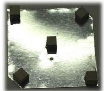
Now its time for a dry fit of the two panels. Align the hole in the element over the SMA's extended post on the reflector. Slide the two parts together so that the SMA's center post passes through the small element panel.
