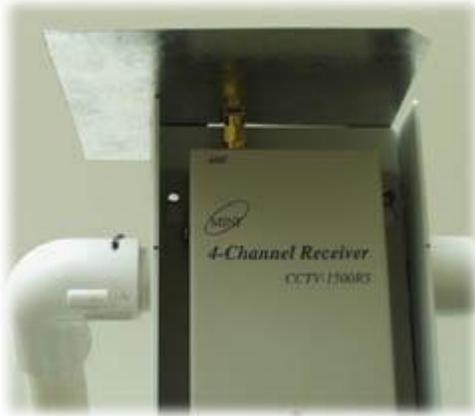
The antenna is now complete! Just screw it onto the SMA of your video receiver and aim it towards your R/C model. The arrow shown on the template is the orientation for use with transmitters with vertical polarization (e.g., vertical Tx whips). If yours is horizontally polarized then rotate the patch 90°.
