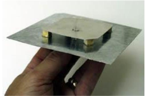
While the glue is drying, solder the SMA's center post to the element. Be very careful or the little wire stub you added will come free from the SMA if its solder reflows. I suggest you solder it while the adhesive is still wet so that you can pull the panels apart if you run into trouble. Cut off the excess wire stub when you are done and allow the adhesive to cure.
