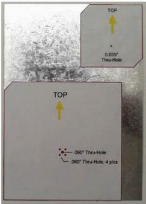
Now cut out the two full scale paper patterns. The red border should be fully intact (cut on the **outside** edge).
